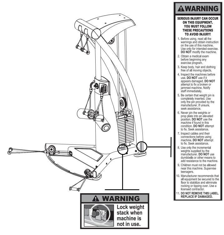
**NOTE:** Lock the weight stack when not using the gym. Make sure all the weight plates are resting on the plate below with no gap in between. Insert the weight selector pin in the tab underneath the weight stack. The weight selector pin should be inserted until the knob touches the metal tab. Once the pin goes through the weight stack system, the weight stack becomes immobile. Verify that the pin has gone through the weight stack stem.
